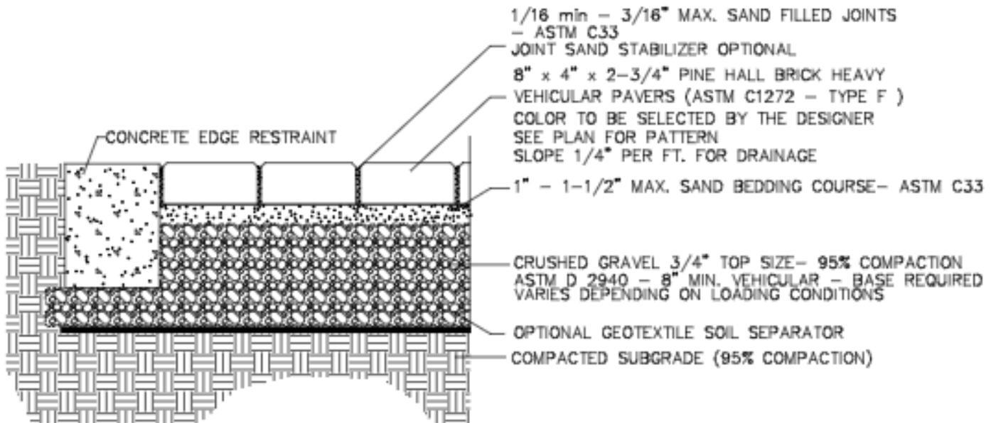
Figure 3: Sand-Set Over Rigid Base CAD Detail
