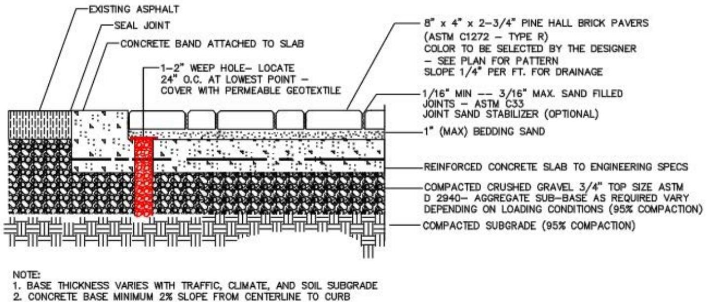
Figure 2: Sand-Set Over Rigid Base CAD Detail
